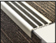
AA346 1 3/8" Right Angle Drop SAFETY STAIR WITH PRE-DRILLED AND COUNDTER-SUNK HOLES FOR #4 SCREW 82° INSERT WIDTH: 13MM X 3 FINISH: EA
