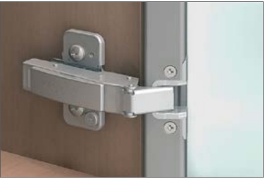
Blum® narrow frame hinge straight arm, 120°, 15mm overlay, self close
