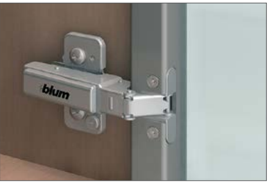
Blum® narrow frame hinge straight arm, 95°, 17mm overlay, self close
